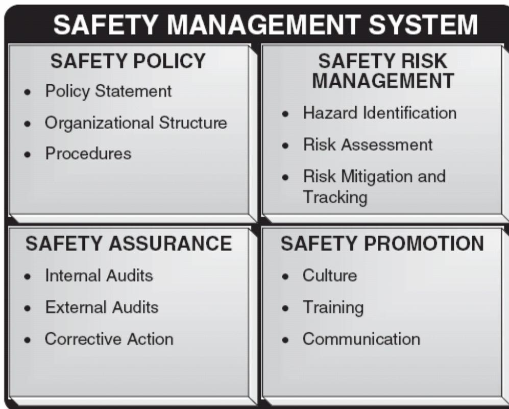
Figure 2: The Pillars of SMS
